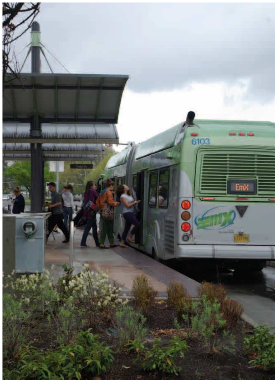
A Bus Rapid Transit station with level boarding (Eugene, OR)
